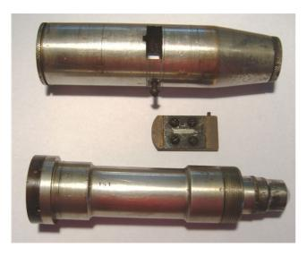
In the photo above, the unusual sound tube (above) is shown contrasted with the standard tube (below) on all portables from their advertised introduction. The slit is also unusual being removable and is pictured between the two sound tubes. It is fitted halfway down the tube in a slot, and held in place by a set screw. The sound tube features six internal condenser lenses which are also of unusual design.
