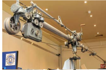
A Mole Richardson telescopic studio microphone boom and cart donated by TVW Channel Seven, Perth.
